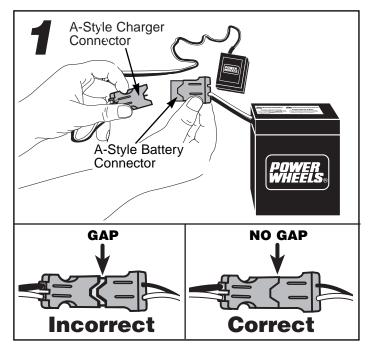
• Plug the charger and battery connectors together. Push firmly to make sure the two connectors are completely joined.
